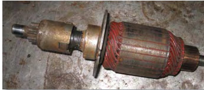
Armature and starter drive from 12-volt 230 civilian starter
